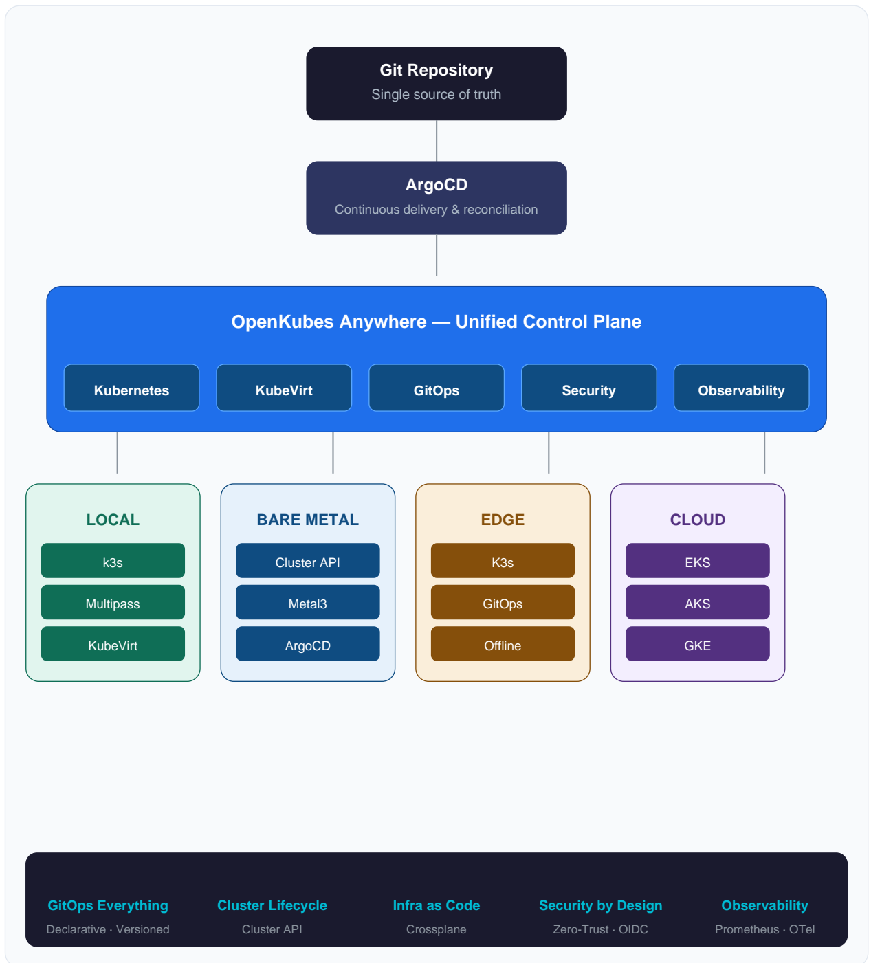
Figure 1: OpenKubes Anywhere platform architecture — Git to workload cluster across all environments
